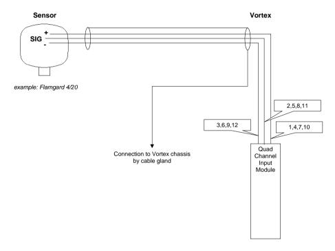
In a system with mixed IS and flameproof sensors in a hazardous area (Zone 1 or 2), the flameproof sensors can be connected as shown above providing the sensor complies with EN50014 and EN50018 (IEC 60079 -0 and IEC 60079 -1).
