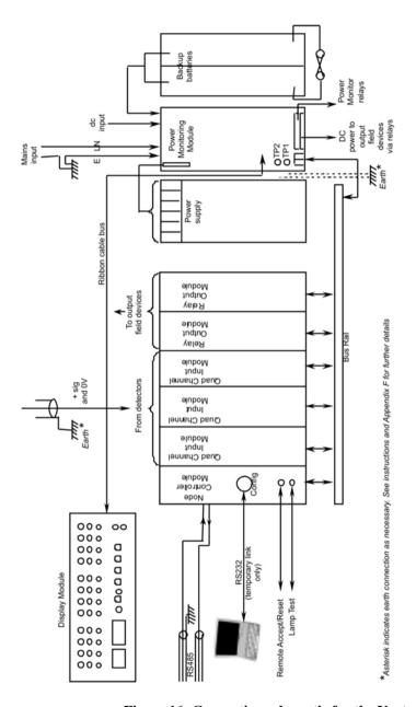
Figure 16: Connection schematic for the Vortex system
