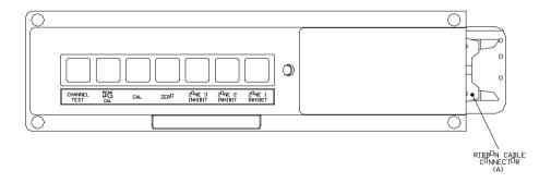
Figure 9: Back of Display Module
