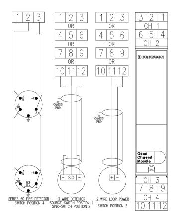
Figure 18: Wiring diagram for the Quad Channel Input Module
