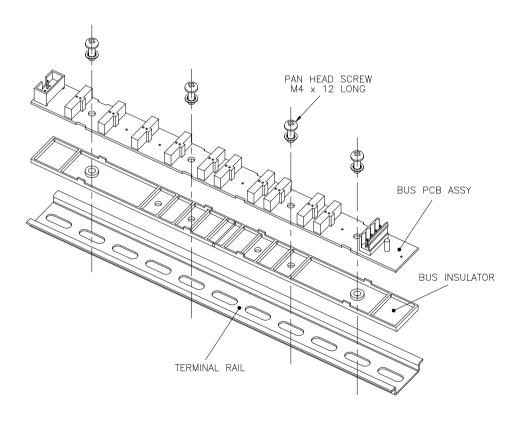
Figure 4: Bus Rail Assembly Details
