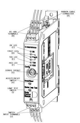
**Figure 3: Node Controller Module**
