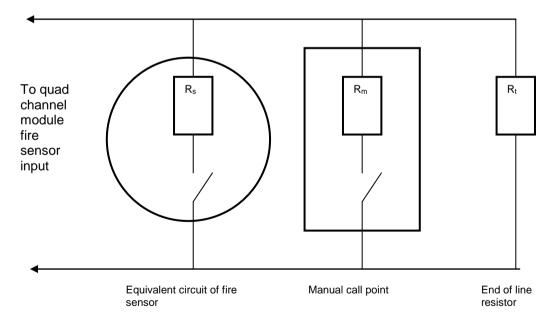
Figure 13: Representation of a fire detection circuit
