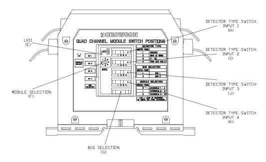
Figure 6: Switches on Quad Channel Input Module
