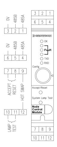
Figure 17: Wiring diagram for the Node Controller Module
