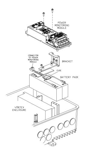
Figure 15: Removing batteries from Vortex Standard Enclosure
