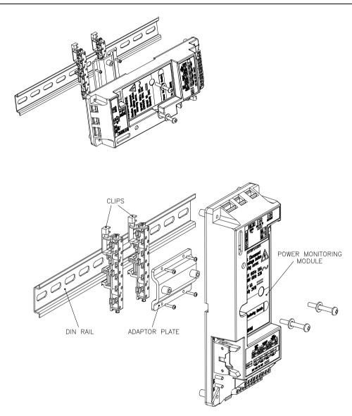
Figure 12: Alternative mountings for the Power Monitoring Module
