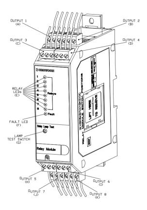
Figure 7: Relay Output Module
