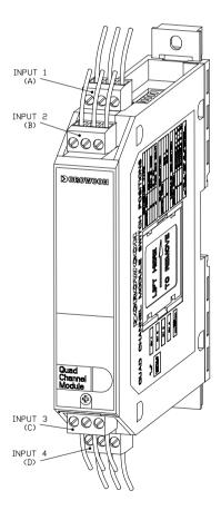
Figure 5: Quad Channel Input Module
