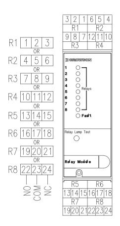
Figure 19: Wiring diagram for the Relay Output Module
