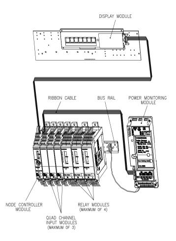
Figure 1: General Assembly of Vortex Modules
