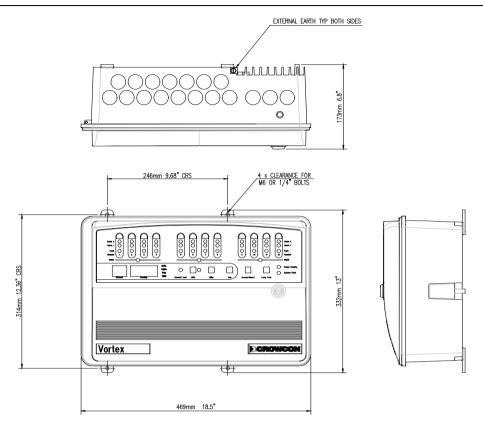
Figure 2: Vortex system in Standard Enclosure
