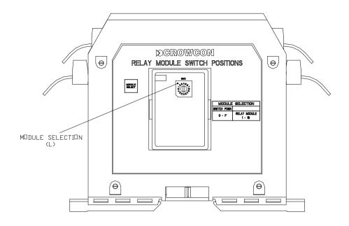
Figure 8: Relay Ouput Module Selection SwitchRelay Output Modules are configured in VortexPC, using the Outputs Configuration option on the Vortex menu. Select the appropriate relay to view its current configuration. The configurable properties of relays are listed in Table 12.
