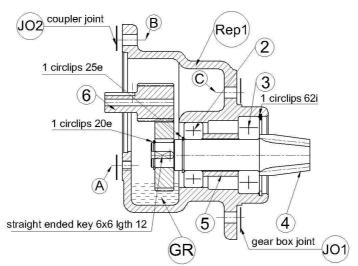
NUTS and BOLTS are assembled using LOCTITE thread-locking product 243
