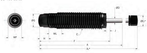
\*Note: A1 and E1 apply to button models and urethane striker cap accessory. One Hex Jam Nut included with every shock absorber.
