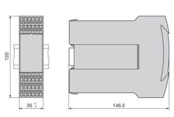
Fig. 6. SINEAX VC 603 in housing **S35** clipped onto a top-hat rail  $(35 \times 15 \text{ mm or } 35 \times 7.5 \text{ mm}, \text{ acc. to EN } 50 \text{ } 022).$
