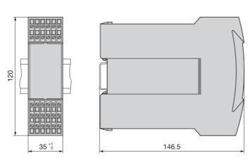
Fig. 6. SINEAX VC 603 in housing **S35** clipped onto a top-hat rail  $(35 \times 15 \text{ mm or } 35 \times 7.5 \text{ mm}, \text{ acc. to EN } 50 \text{ } 022).$
