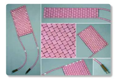
The cold tails of Cooperheat ceramic heating elements are butt welded to the heater core wire which eliminates the cold tail/core wire junction failures often seen with low quality heaters which use steel ferrules.
