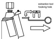
Extract the clip putting the extraction tool (KM/3062) in the hole of the security clip then pull hard to extract the clip.
