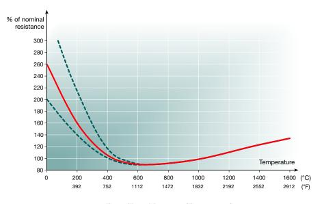
Fig. 4 Typical Resistance/Temperature Curve
