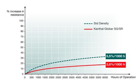
Fig. 3 Typical change in resistance with time at 1400°C (2552°F) (Continuous operation in an air atmosphere)
