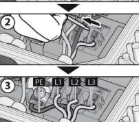
Fig. 2: Connecting wires to terminals
