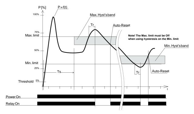
The Figure above shows a typical AC-motor power consumption curve immediately after power has been applied to the motor. The bars at the bottom of the figure indicate power applied to the unit and the position/state of the relay (On/Off). The figure shows the functions
