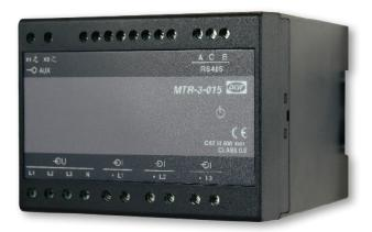
The size of a portable hard drive, the MTR-3 transducers are slight in build but offers equal performance of up to four standard transducers, measuring and calculating AC voltage, AC current, active/reactive/apparent power, power factor, frequency, kWh, kVAr, THD, dynamic and maximum demands.
