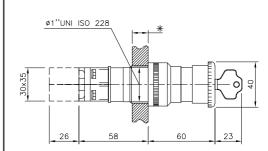
DFP 5 / DFP 8 Normal /With lock (press and pull) Weight = 280 g / 280 g
