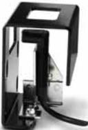
Heavy-duty bracket protects the sensor from damage. Works with all OEM Prism Series sensors. Ideal for material handling applications with the OEM Prism Series right angle polarized reflex sensor. Provides locking vertical and horizontal adjustments for independent adjustment in each axis. Sensor mounts on #4 studs. 10 ga. painted steel | <b>E58KS5200</b>                       |
