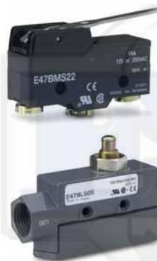
Precision switches are typically available in two types: basic precision and enclosed precision. The basic precision switch is of one-piece construction. The enclosed precision switch is simply a basic switch inside a die cast housing. Basic precision switches are generally not given a NEMA enclosure rating, while some enclosed precision switches can be rated NEMA 4 or 13.
