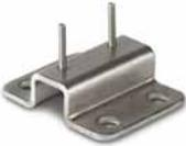
Contoured design is ideal for flush mounting of right angle OEM Prism Series polarized reflex to mounting surface using 1/4 in hardware. No alignment adjustment. Sensor mounts on #4 studs. 304 stainless steel                                                                                                                                     | <b>6161AS5296</b>                      |
