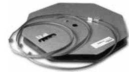
The buss harness distributes power, slug release signals and provides communications links. Made from flat ribbon cable, it is available in 10, 50 and 100 ft lengths and is connectorized at intervals to match your zone length (18 to 60 inches in 6 inch increments).
