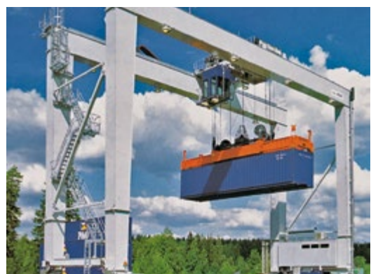
Rubber tyred Gantry crane.
