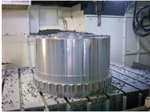
Machining hub TCB-HD-10200.
