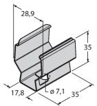
Snap bracket for mounting WLS28 work lights
