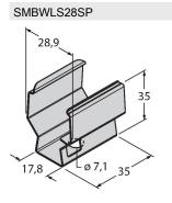
Snap bracket for mounting WLS28 work lights
