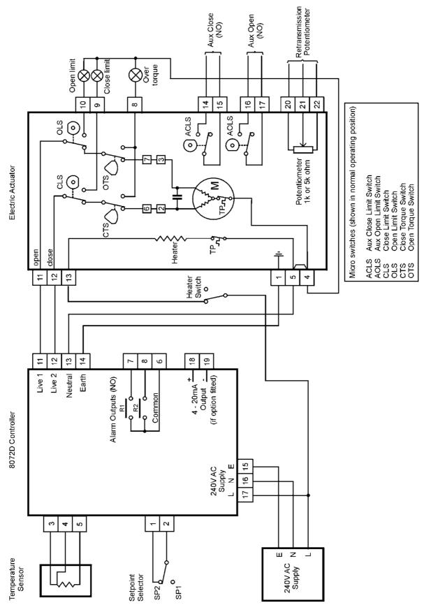
Fig 13 System Wiring Diagram 8072D Controller
