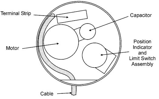
*Fig 5 Actuator Internal Cable Routing*
