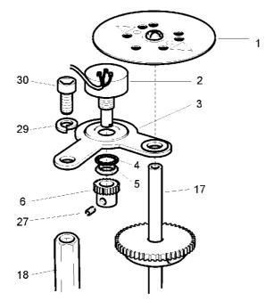
Fig 8 Potentiometer Assembly
