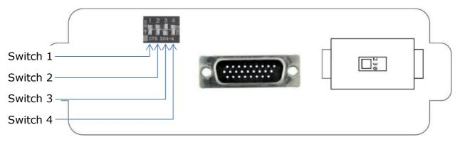
Fig 6 Positioner Switch Location
