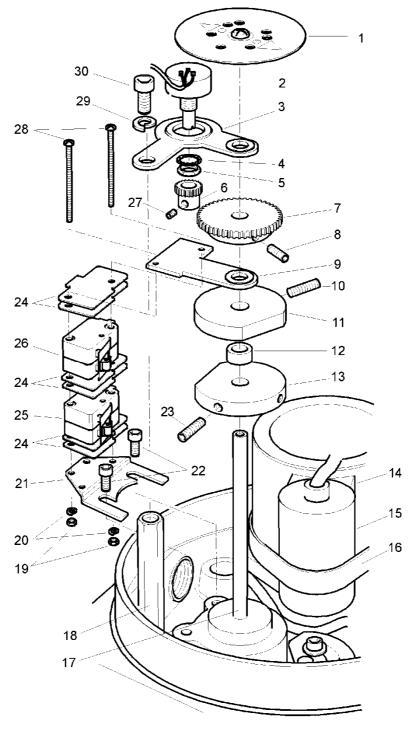
Fig 7 Limit Switch assembly
