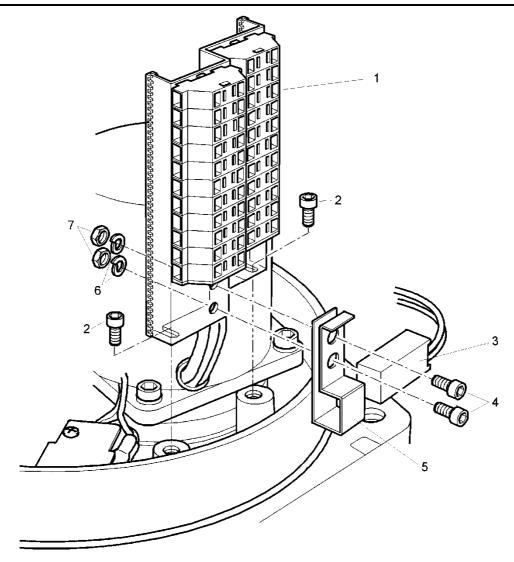
Fig 10 Anti-Condensation Heater
