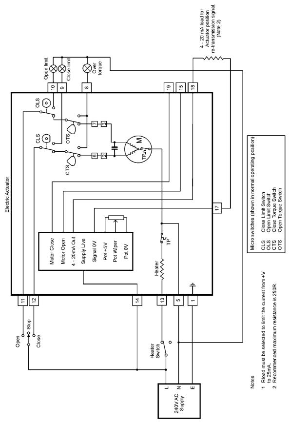
*Fig 15 System Wiring Diagram Electronic Positioning Unit switched mains voltage input*
