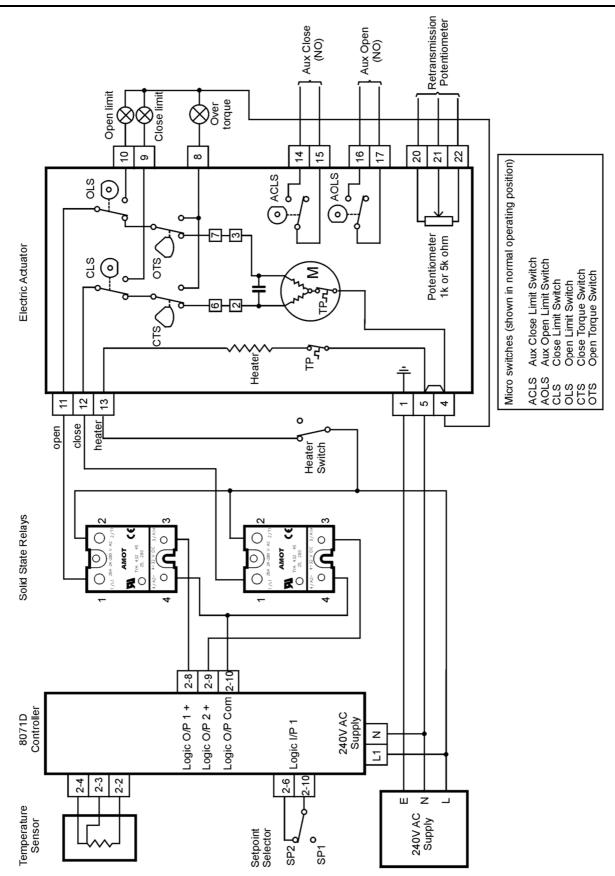
Fig 11 System Wiring Diagram 8071D Controller with two Solid State Relays
