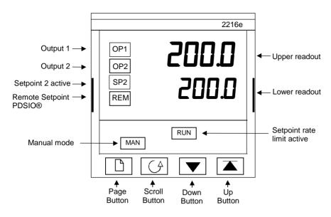
Fig 1-1 Model 2216e front panel layout
