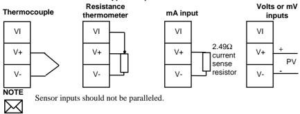
Fig 2-7 Sensor input connections
