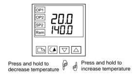
Figure 1.5 The lower readout shows the setpoint
