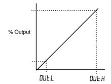
For output of 0-100% = 0-20mA set DuE H to 20.0 and DuE L to 0.0
