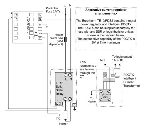
Figure E.1 Connections for Mode 1 & 2
