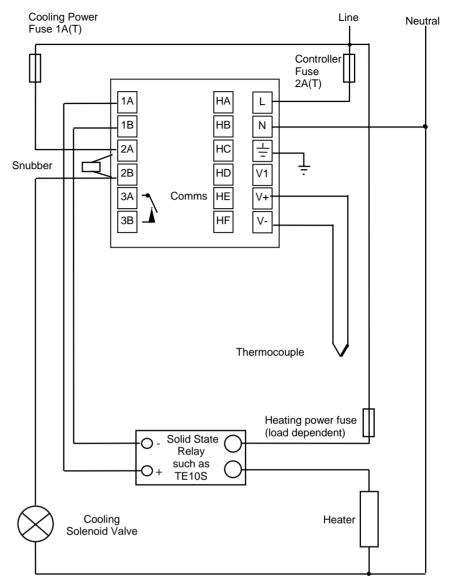
Fig 2-8 Typical wiring diagram, Model 2216e Controller
