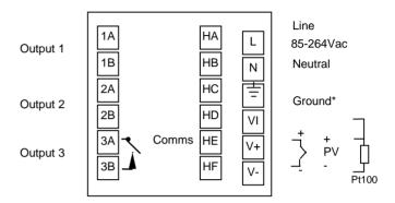
Figure 2-3 Model 2216e wiring connections
