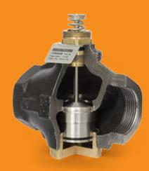
2TBB Series = 2-way valves, bronze body, with threaded connections up to 2", brass plug, stainless steel stem. Temperature applications -10°C to 130°C. Rangeability 50:1. To be motorised by MVE and MVH actuators (no adapter needed).
