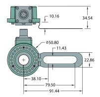
All dimensions are in mm with a tolerance of ±0.127mm or ±0.254mm unless otherwise specified
