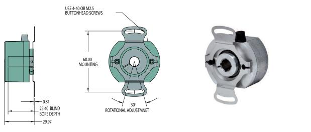
All dimensions are in mm with a tolerance of  $\pm 0.127$  mm or  $\pm 0.254$  mm unless otherwise specified
