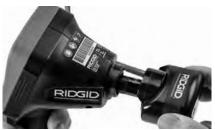
Figure 18 - Camera Connector Plug Installed
