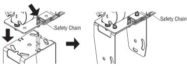
Mounting Safety Chain to a Compact Oil Damped Bracket
