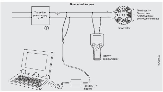
RL = Load resistance for HART® communication RL min. 250  $\Omega$ , max. 1,100  $\Omega$
