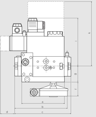
d = Space requirement for cover of pressure switch
