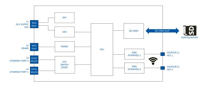
The vCOM interface has an Ethernet-based interface for connecting to the management (stationary side) and/or to the subordinate IO devices (mobile side). The SMGM and SMGX are optimized for both PROFINET-IO and PROFIsafe transmission.
