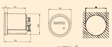
type 587/60.1  $\dots$  2 type 588/60.1  $\dots$  2 with damping rubber
