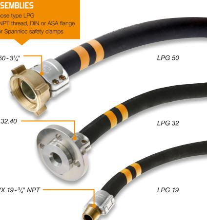
For bulk refueling we recommend our LPG hoses to EN 1762, sizes DN 10 to 200 mm. The hose construction with braided reinforcements gives them an unequalled combination of flexibility, pressure safety and long service life. End fittings (ACME/NPT thread, DIN/ASA flanges) of steel, stainless
