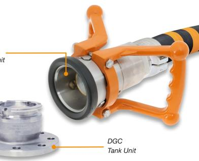
steel or brass are assembled with reusable SPANNLOC or SPANNFIX safety clamps. WP PN 25 - test presure 40 bar - burst pressure >100 bar.
