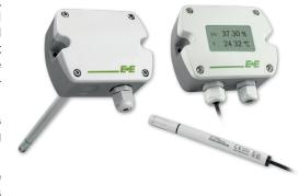
With an optional USB configuration adapter, the user can set the RS485 interface parameters, the output scaling and perform one or two point adjustment for RH and T.
