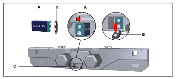
Figure 16 Connecting the nine-volt battery
