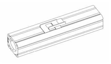
2) Assemble the second bracket facing opposite the first, with one leg going in between the legs of the first bracket as shown above.
