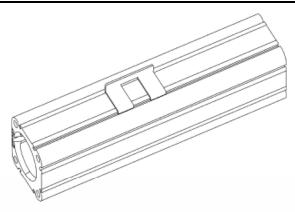
1) Choose which of the available barrel sides you want to mount your switch. Assemble one bracket with its two "claws" going inside the barrel groove as shown above.
