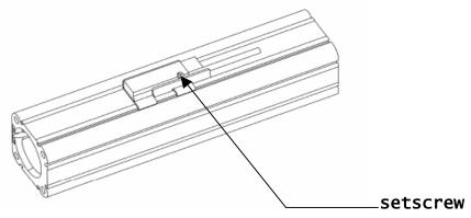
3) Slide the switch into place (between the brackets) as shown. Locate brackets & switch at the point along the barrel where actuation is desired. Tighten the setscrew with the Allen key furnished.
